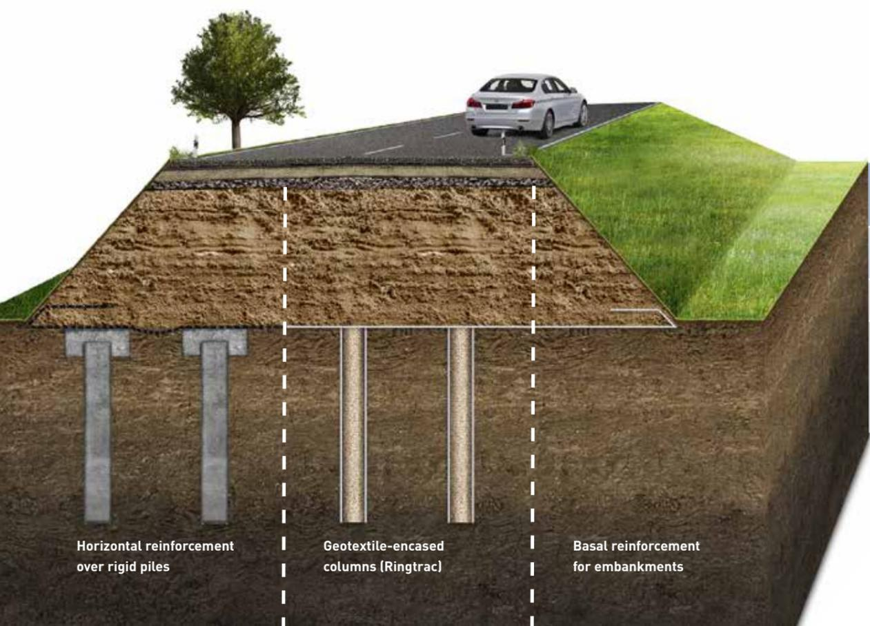
Horizontal reinforcement over rigid piles
